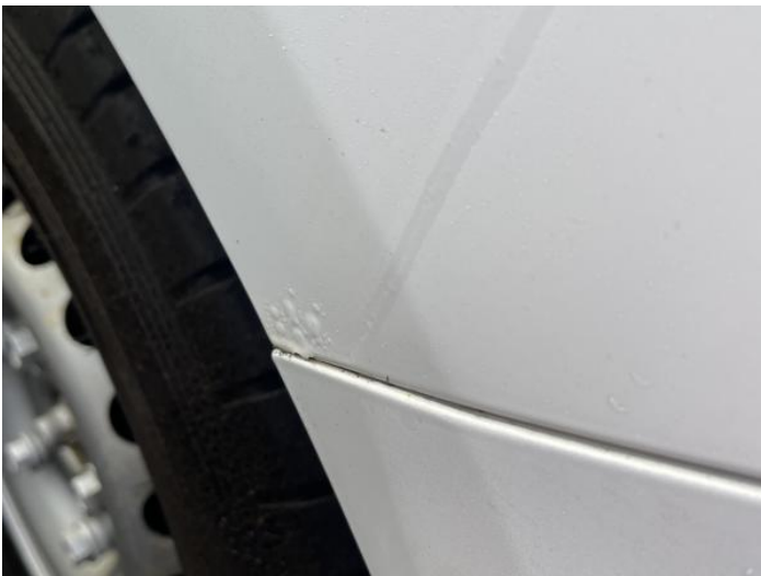
1: Wing osf Rusted Over 5mm
