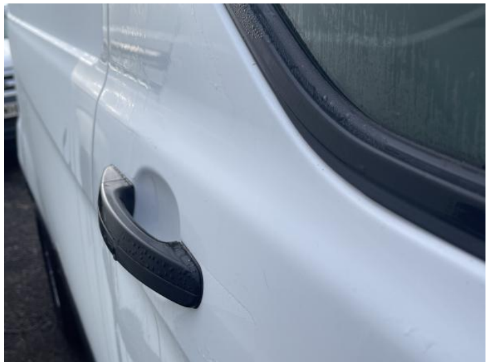
2: Door osf Dented Over 2 UpTo 10mm
